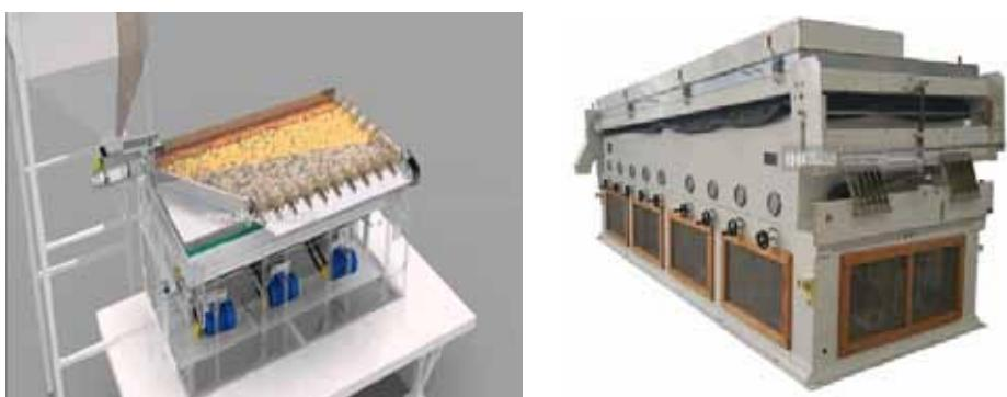
Fig : Gravity Separator
